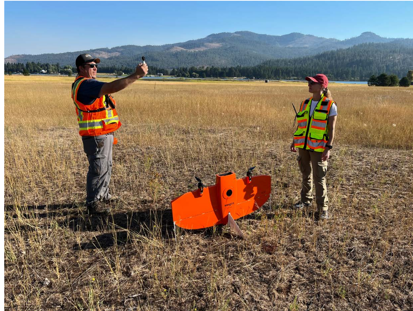
USACE Small Unmanned Aircraft System crew checking wind speed and direction prior to aerial drone survey of archaeological sites at the Albeni Falls Dam Operating Project, ID. (Jacques Kerkhove-Peltier/USACE)
