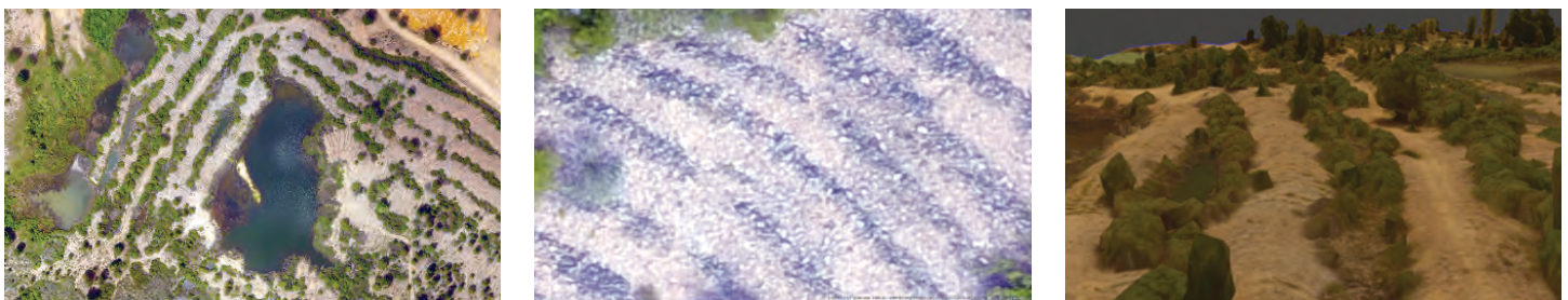
Figure 6. From left to right: dredge tailings captured with drone, scale 1:1,000; orthomosaic image of Idaho City Mining District, scale 1:50; the 3D Model Generated in Pix4D using Drone Imagery. (Courtesy images by Northwest Nazarene University)
