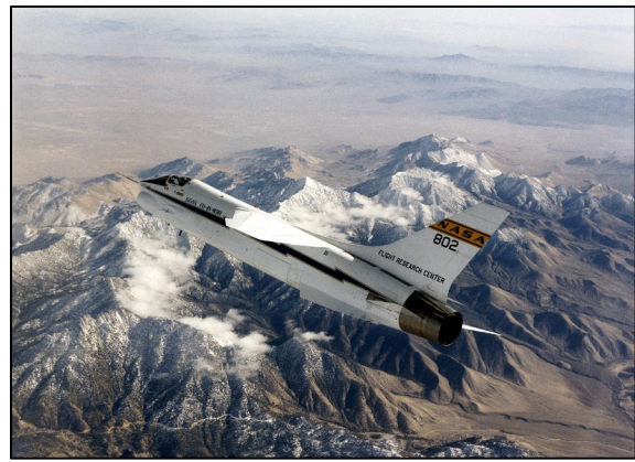
Figure 3-1. The success of NASA's F-8C "Digital Fly-by-Wire" Program (1969-1985) resulted in the adoption of digital flight controls, now standard in aircraft.
