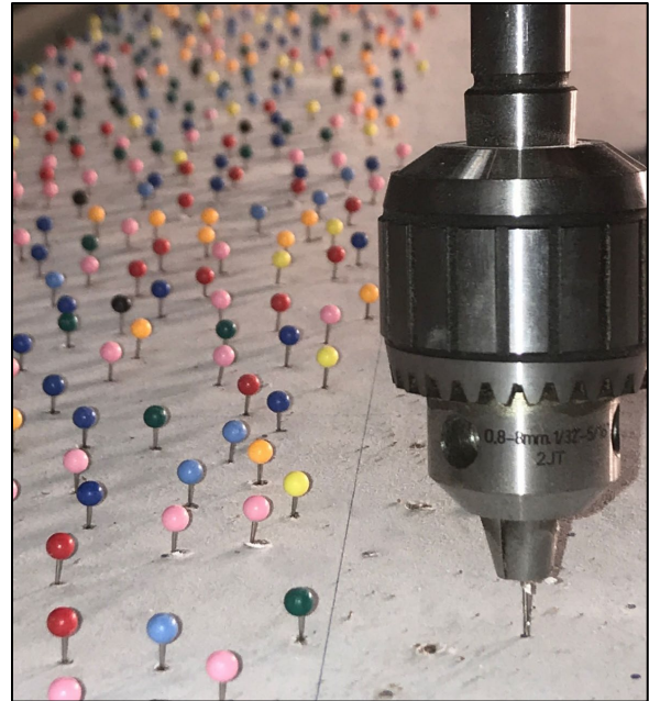
Figure 4-6. Ceiling tile stamping technique employed to replicate the original.
